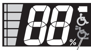
Varsellampe for "Tilbaketrunket tippesikring"
