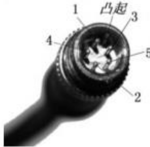
Panel Outlet Terminal
